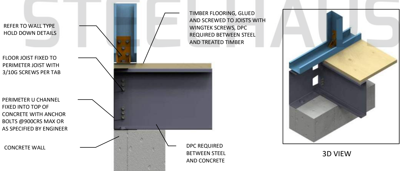
MIDFLOOR PERIMETER CHANNEL FIXED OVER CONCRETE WALL
