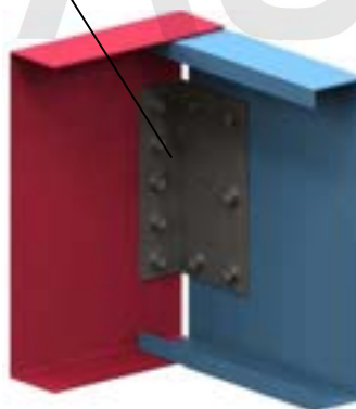
TYPICAL END EJ TO EP BRACKET CONNECTION
